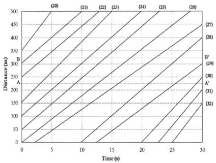
i) An observer recorded the times at which the front end of the vehicles passed sections A-A' and B-B' and the data were noted as shown in the table below. Based on the information provided in both the table and time-space plot, determine the space mean speed (in km/h) of the vehicles travelling within the section A-A' and B-B'
