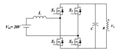
The switches  $S_1$  and  $S_4$  are turned-on at the same instant and are in conduction for 30  $\mu$ s, while  $S_2$  and  $S_3$  are turned-on at the same instant and are in conduction for 20  $\mu$ s. The switching frequency of the devices is kept at 20kHz. Assume the switches are ideal and the converter is lossless.  $C = 2 \, mF$ ,  $R = 100 \, \Omega$ ,  $L = 2 \, mH$ .
