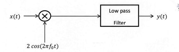
where the lowpass filter is an ideal filter with a cut-off frequency of W Hz. If the spectrum X(f) of the input signal x(t) is as shown in the figure below, determine and sketch the spectrum of the output signal y(t).
