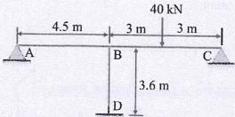
8. (a) For the cantilever beam, determine the vertical deflection at point A using stiffness method. Also, determine the fixed end moment at B and draw BMD. (15)
